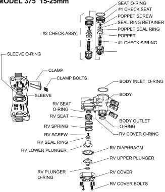
When the relief valve discharges intermittently, it can be almost always assumed that the device is functioning correctly and that the discharge is caused by system problems such as inlet pressure fluctuations or water hammer due to quick closing valves
