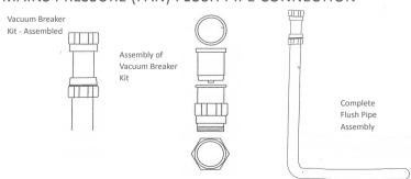
Please note: Turn tube nut onto flush valve body hand tight plus 1/8th turn. Over tightening will damage vacuum breaker and void warrantry
